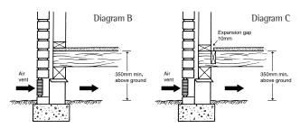
CONSTRUCTION PLATFORM FLOORING – Methods described generally apply to Platform Construction (refer to diagram B) or AS/NZS1860 Section 7 for further details. Although an exposure period of 3 months maximum is permitted, efforts should be made to protect FLOORBOARD from excessive exposure. Any ponded water
