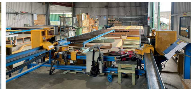
Above left: Infeed leading to the computerised Razor 5 saw, supplied by Vekta. Above right: FrameQuip frame line, which has been a welcomed addition particularly with the improvements seen in safety.
