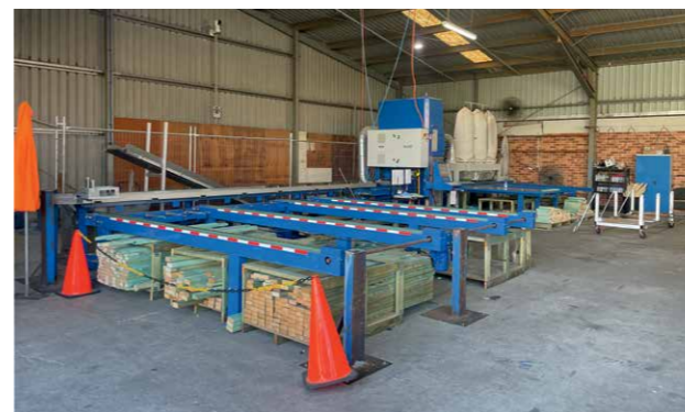
Above left: Infeed leading to the computerised Razor 5 saw, supplied by Vekta. Above right: FrameQuip frame line, which has been a welcomed addition particularly with the improvements seen in safety.
